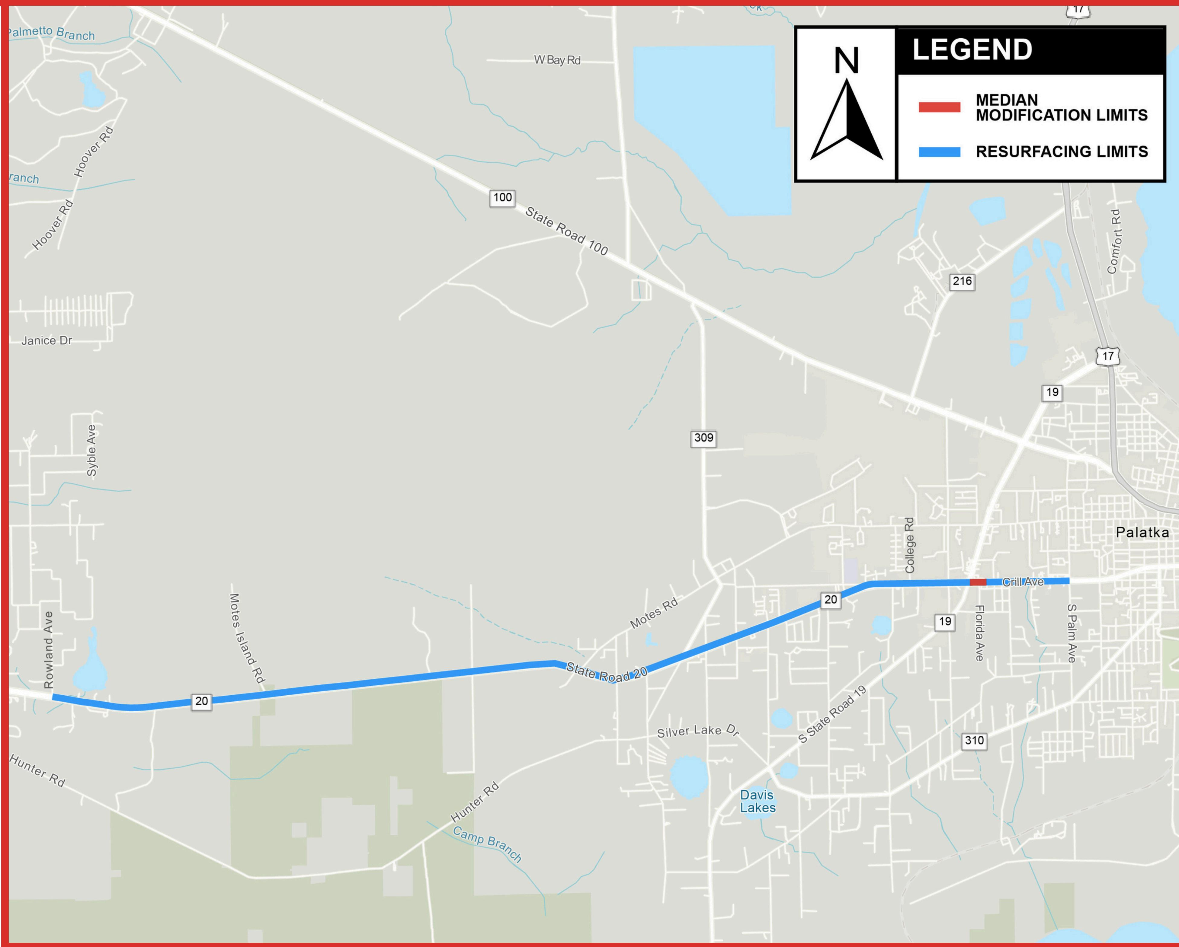
The project includes resurfacing, restoration and rehabilitation along State Road 20 (Crill Avenue) from Rowland Avenue to South Palm Avenue. Work will include milling and resurfacing the roadway.
